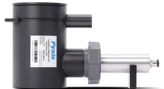
Figure 11. L-CAL Liquid Turbidity Calibration Kit (P/N 53247)
